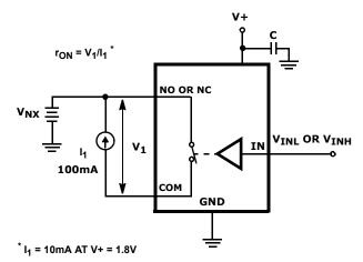
FIGURE 5. ron TEST CIRCUIT
