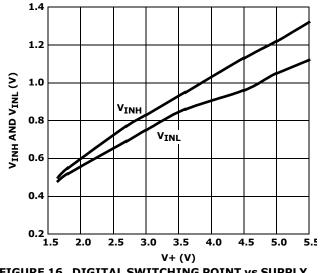
FIGURE 16. DIGITAL SWITCHING POINT vs SUPPLY VOLTAGE
