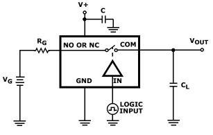
**FIGURE 2A. MEASUREMENT POINTS**
