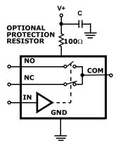
FIGURE 8. V+ SERIES RESISTOR FOR ENHANCED ESD AND LATCH-UP IMMUNITY
