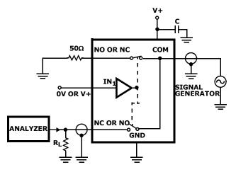
FIGURE 6. CROSSTALK TEST CIRCUIT
