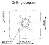
Soldering pad geometry
