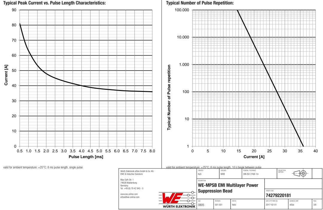
**Typical Peak Current vs. Pulse Length Characteristics:**
