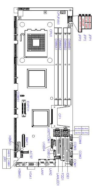
**Board Layout: Jumper and Connector Location**
