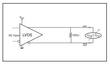
**Differential Output Voltage Setup**
