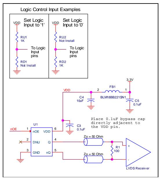
Figure 2. IDT8N4S273 Schematic Example
