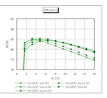
Fig.12-3-8. Efficiency v.s. Output Current
