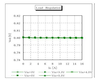
Fig.12-3-7. Output Voltage v.s. Output Current
