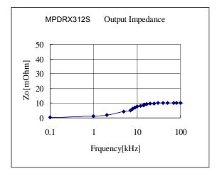
Fig.12-2-1. Output Impedance of MPDRX312S
