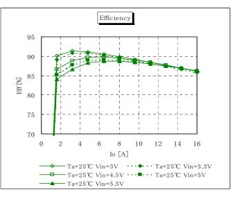
Fig.12-3-2. Efficiency v.s. Output Current
