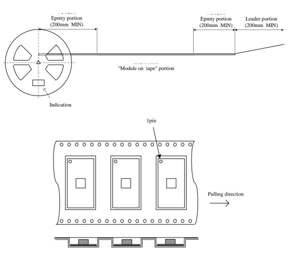
The module is located such as parts in upper side and PCB in lower side.
