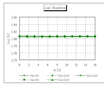
Fig.12-3-1. Output Voltage v.s. Output Current
