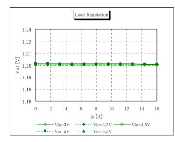
Fig.12-3-4. Output Voltage v.s. Output Current
