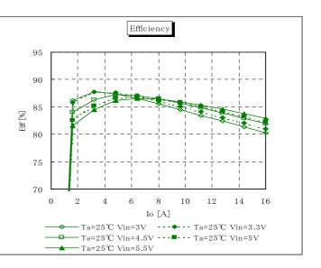
Fig.12-3-5. Efficiency v.s. Output Current
