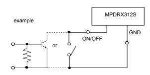
..... Output Voltage =ON ..... Output Voltage=OFF
