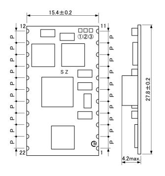
( )…reference value P=2.54 ±0.2mm Tolerance is not accumulated.
