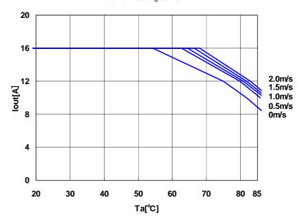
The above derating limits apply to this product soldered directly to 101.6\*180mm\*1.6mm PCB. Any adjacent parts of high temperature may cause overheating. For reliable operation, please ensure that the FET temperature of this product is maintained below 120°C and the inductor temperature is below 106°C.
