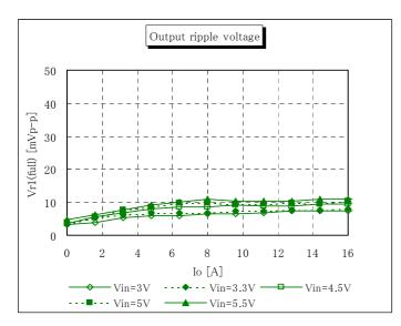
Fig. 12-3-3. Ripple Voltage v. s. Output Current
