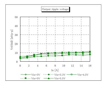
Fig.12-3-6. Ripple Voltage v.s. Output Current
