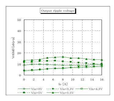
Fig.12-3-9. Ripple Voltage v.s. Output Current
