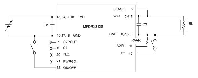
$\begin{array}{lll} C1:100\mu F/6.3V & Ceramic Capacitor\\ C2:100\mu F/6.3V & Ceramic Capacitor\\ Please make sure to place C1 and C2 nearby input and output terminal of DC-DC converter.\\ \end{array}$
