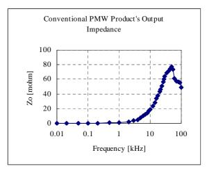
Fig.12-2-2. Output Impedance of conventional product
