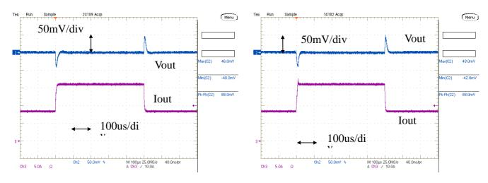
Fig.12-1a. Load Transient Response (Vout:1.8V)
