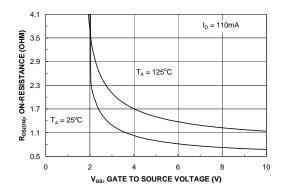
Figure 4. On-Resistance Variation with Gate-to-Source Voltage.
