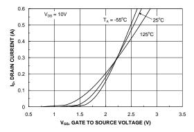
Figure 5. Transfer Characteristics.
