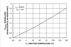
Figure 3. On-Resistance Variation with Temperature.
