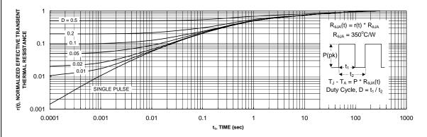
Figure 11. Transient Thermal Response Curve.
