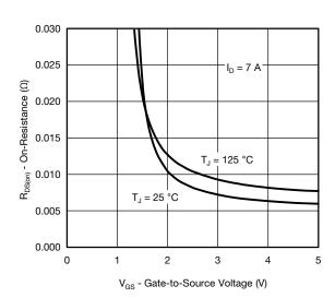
On-Resistance vs. Gate-to-Source Voltage
