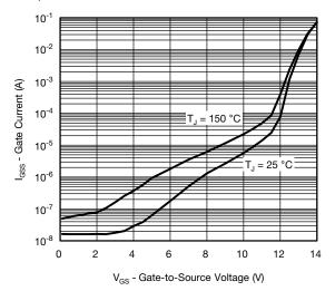
Gate Current vs. Gate-Source Voltage
