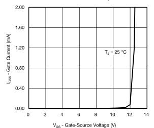
Gate Current vs. Gate-Source Voltage
