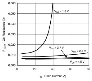
On-Resistance vs. Drain Current and Gate Voltage
