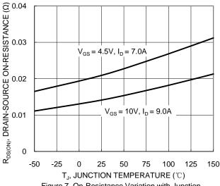
Figure 7. On-Resistance Variation with Junction Temperature
