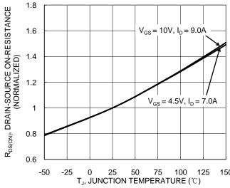
Figure 6. On-Resistance Variation with Junction Temperature
