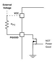
Figure 45. PGOOD Block Diagram
