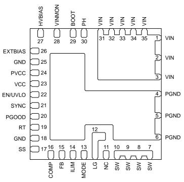
Figure 3. Pin Assignment (Bottom View)
