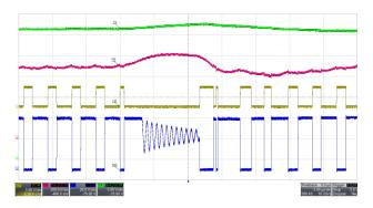
Figure 32. OVP2 at  $V_{FB} \ge 130\% V_{REF}$
