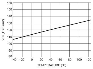
Figure 12. EN/UVLO Hysteresis Voltage vs. T at V<sub>HVBIAS</sub> = 48 V
