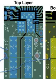
Place some vias on the VIN and PGND pads right under the device
