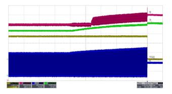
Figure 30. OVP1 at V<sub>FB</sub> ≥ 115% V<sub>REF</sub>
