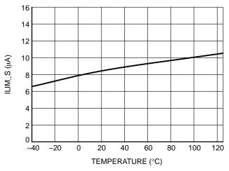
Figure 20. 8.5  $\mu$ A Current Source for Current Limit Purpose vs. T at  $V_{HVBIAS}$  = 48 V
