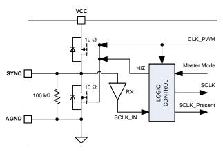
Figure 44. Frequency Synchronization Block Diagram
