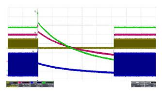
Figure 33. OVP2 Release at  $V_{FB} \le 100\% V_{REF}$
