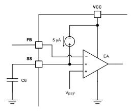
Figure 42. Soft Start Block Diagram
