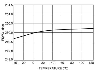
Figure 15. Switching Frequency vs. T at  $V_{HVBIAS}$  = 48 V and RT shorted to  $V_{CC}$
