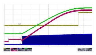
Figure 28. Power Good at Startup with No Load
