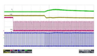
Figure 25. Transition from Native Frequency to Sync Frequency in Non-Master Mode
