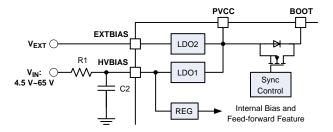
Figure 40. LDO Block Diagram
