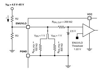
Figure 41. EN/UVLO Block Diagram
