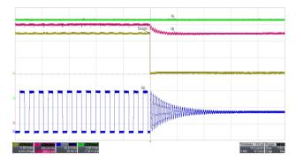
Figure 29. Power Good at Startup with No Load
