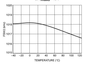
Figure 14. Switching Frequency vs. T at  $V_{HVBIAS}$  = 48 V and RT = 8.06 k $\Omega$
