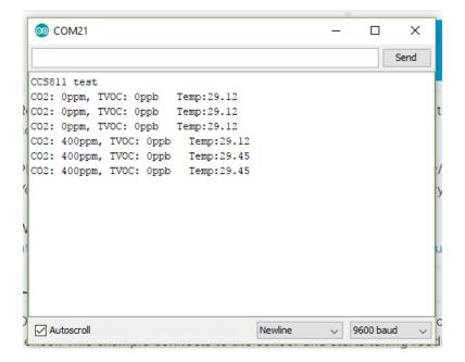
AMS recommends that you run this sensor for 48 hours when you first receive it to "burn it in", and then 20 minutes in the desired mode every time the sensor is in use. This is because the sensitivity levels of the sensor will change during early use.
