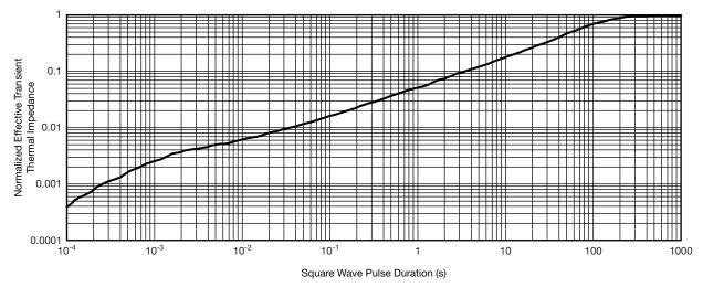
Normalized Thermal Transient Impedance, Junction-to-Ambient
