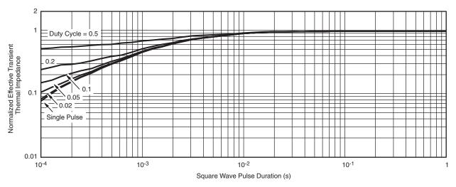
Normalized Thermal Transient Impedance, Junction-to-Case
