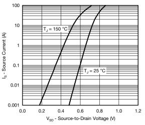
**Source Drain Diode Forward Voltage**
