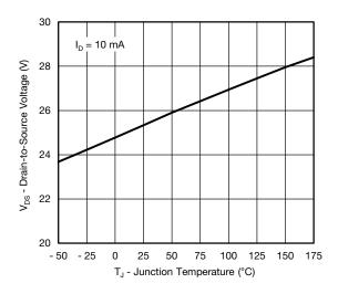
**Drain Source Breakdown vs. Junction Temperature**
