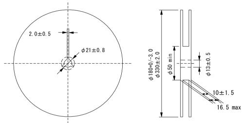
Fig.3 Taping Diagram
