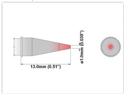
EP75C010 Conical 1.00mm (0.04")
