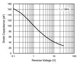
Fig. 6 - Diode Capacitance vs. Reverse Voltage
