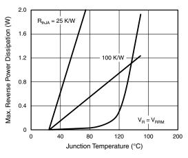
Fig. 5 - Max. Reverse Power Dissipation vs. Junction Temperature
